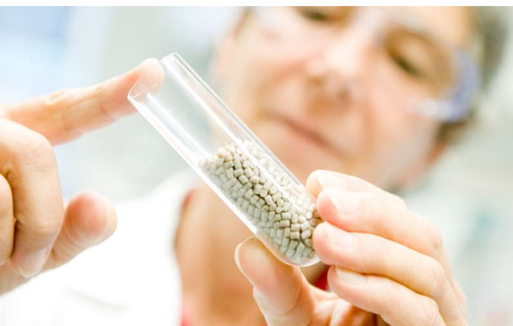
A polyetheretherketone (VESTAKEEP PEEK) sample is checked in the laboratory before being dissolved and analyzed.
