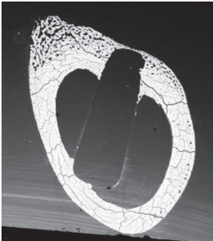
Fig. 2. Transparency to x-rays is a benefit of PEEK implants, since in contrast to titanium implants will grow inside the implant can be confirmed
